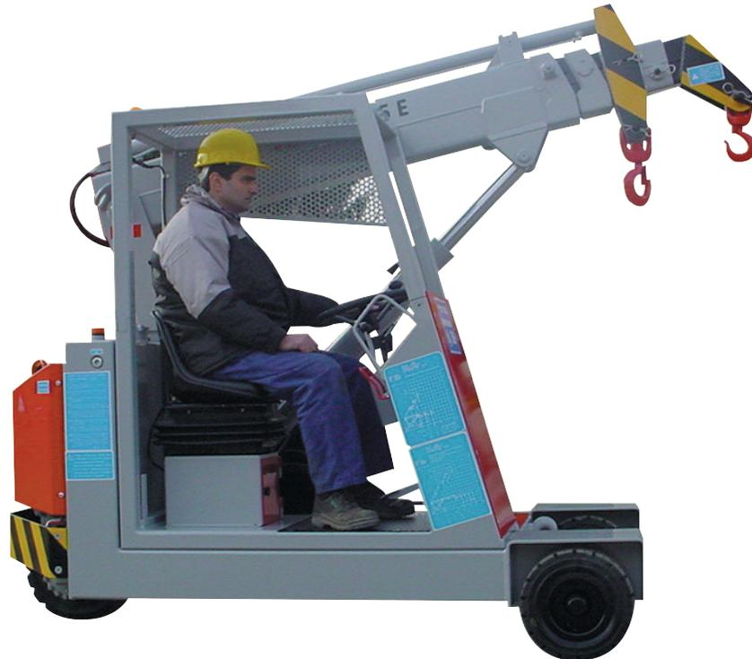
**DRIVE:** DC 3.3 kW - 24 V fanned reversible electric motor with MOSFET electronic control HF and energy saving, self diagnostic, speed and temperature checks (no. 2 thermostats), brush wear warning. Foot hydraulically operated brake to drive wheel. Hand brake mechanically operated. Gear box between motor and drive wheel in oil bath. Speed up to 8 km/h.
